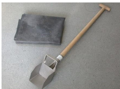
Figure 1: sampling trowel handshaft
