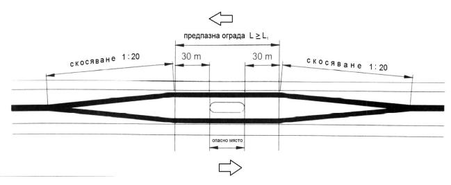
Figure 19. Formation of a road restraint system at a hazardous location in a median dividing strip
