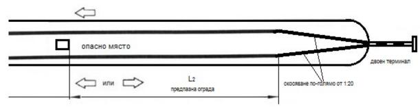
Figure 22. Restraint system built bilaterally in a median dividing strip of one-sided road restraint system with two-sided terminal as a start
