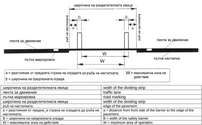
Figure 17. One-sided road restraint system for split-action roads located to the edge of the
