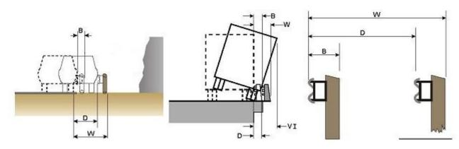
Figure 1. Area of operation (W), zone of normed encroaching of the vehicle into an unprotected area (VI), dynamic deformation of the barrier (D) and width of the barrier before impact (B)
