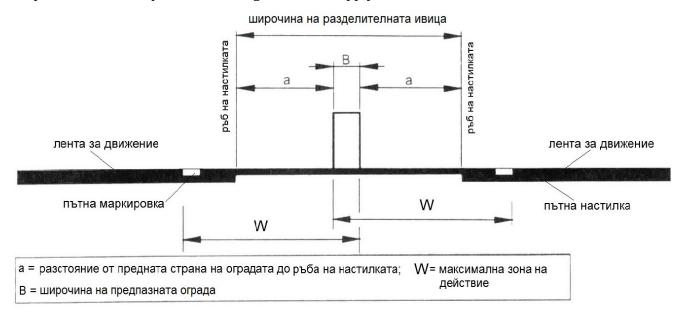
Figure 15. Two-sided road restraint system located in the axis of the dividing strip
