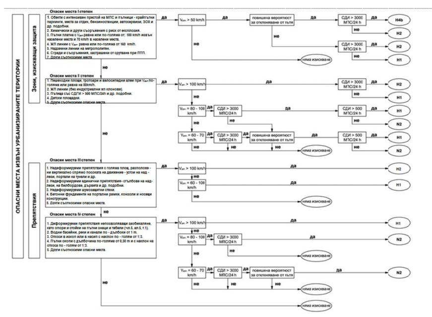
Figure 3. Algorithm for determining the retention rate of a restraint system for roads outside the urban areas
