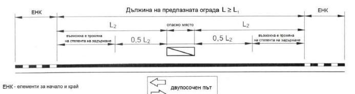
Figure 4. Minimum length of a road restraint system on a two-way road
