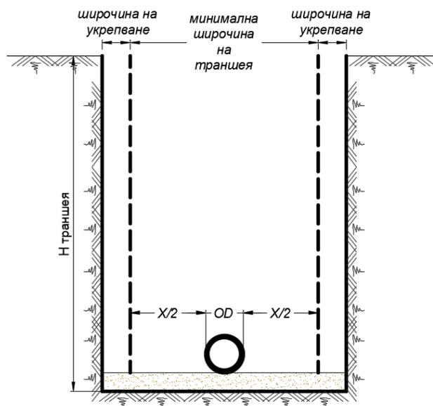
**Figure 1 Strengthened trench**
