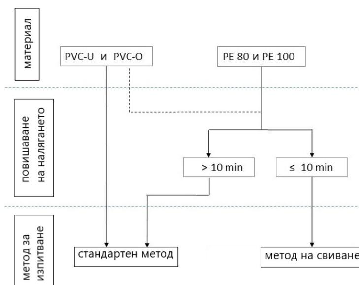
**Figure 9 – Choice of the test method**
