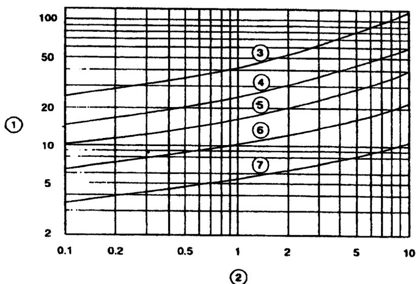
Relation between the dimensioning value of the roughness  $k_2$  and pressure losses at different internal diameters  $D$  (for water supply section with a length of 100 m, water velocity of 1.5 m/s and water temperature of  $10^\circ\text{C}$ ): 1 – pressure losses, kPa; 2 – roughness,  $\text{m} \times 10^{-3}$ ; 3.  $D = 100$  mm; 4.  $D = 150$  mm; 5.  $D = 200$  mm; 6.  $D = 300$  mm; 7.  $D = 800$  mm
