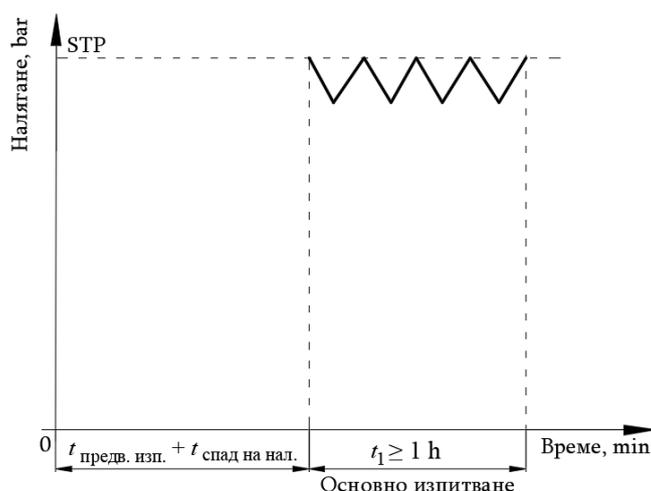
**Figure 3 – Diagram of the test process using the water loss method by measuring the pumped volume of water**
