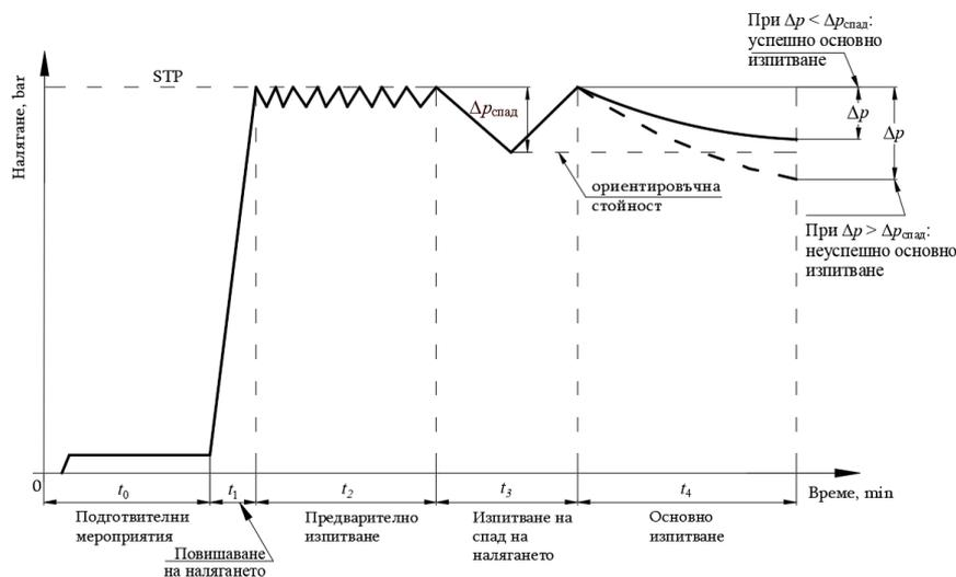
Figure 1 – Test stages for pressure loss method
