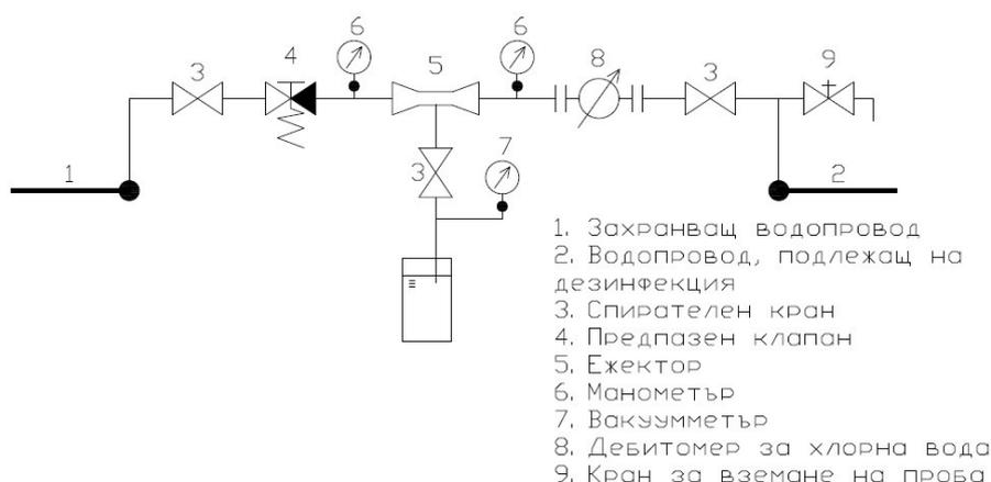
Figure 1. Installation for disinfection with ejector
