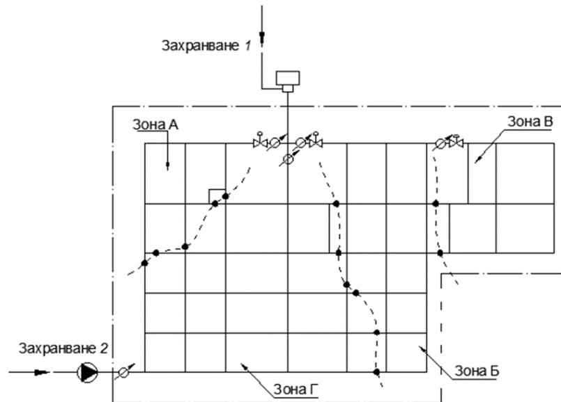
**Figure 1 Water supply network, which is divided into zones by boundary stop taps (areas A, B and C have one power supply and zone D has two power supplies)**
