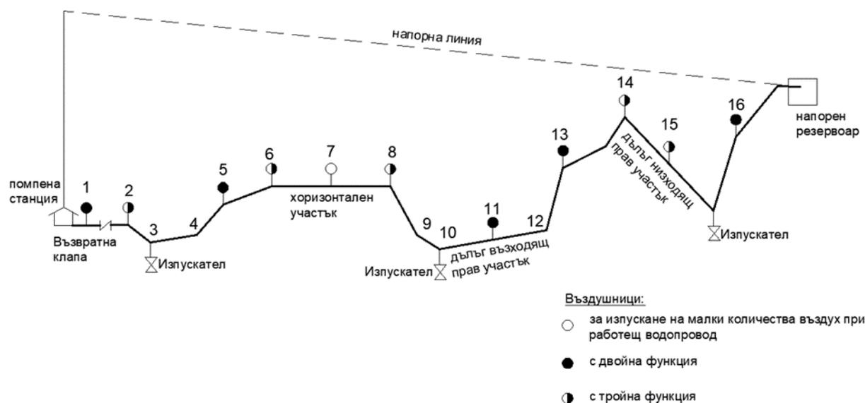
**Figure 1 Example positioning of different types of air vents in thrusting plumbing after a pump**
