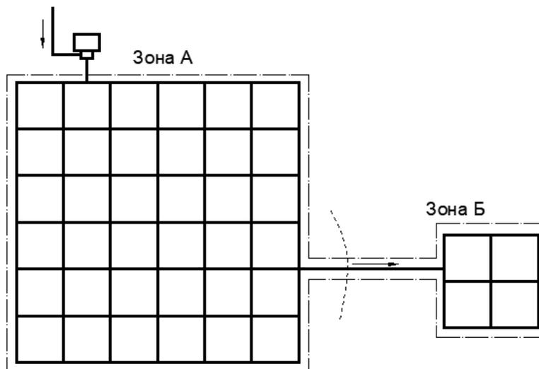
**Figure 3 Zoning of the water supply network of a settlement with a separate urbanized area (e.g. remote residential complex)**
