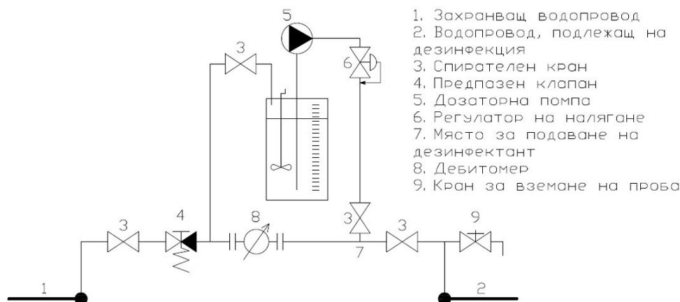
Figure 2. Disinfection instalation with a dispenser pump
