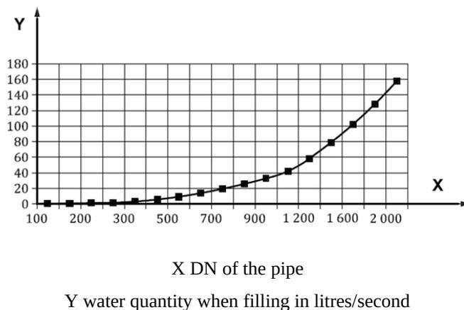
**Figure 5 – Typical water quantities when filling**
