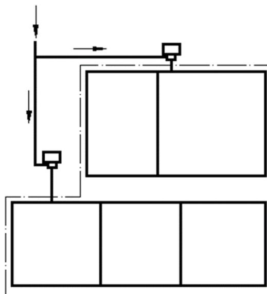
**Figure 2 Water supply system divided into two zones, each of which has independent water supply**
