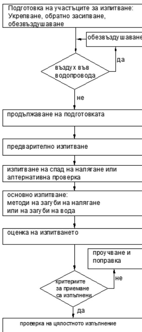
**Figure 2 – Block diagram of the pressure test procedure**
