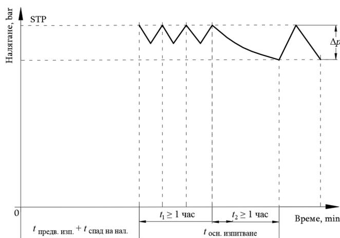
**Figure 2 – Test process using the water loss method by measuring the drained volume**
