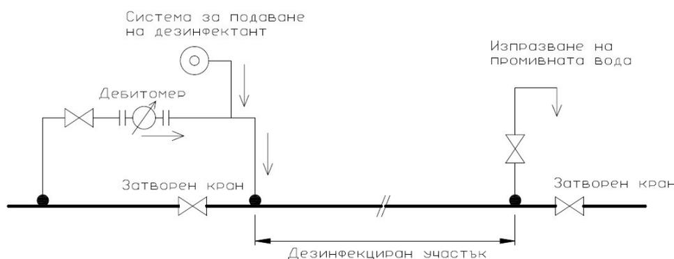
Figure 4. Installation for disinfection of a pipe section using the water and the pressure of the water supply network
