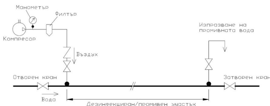
Figure 3. Hydropneumatic flushing installation
