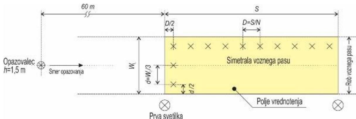
Figure 46: Placement of measuring points in each lane for luminance measurement
