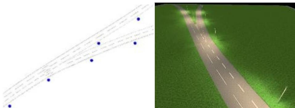
Figure 18: Example of the placement of lamps for the lighting of the expressway junction
