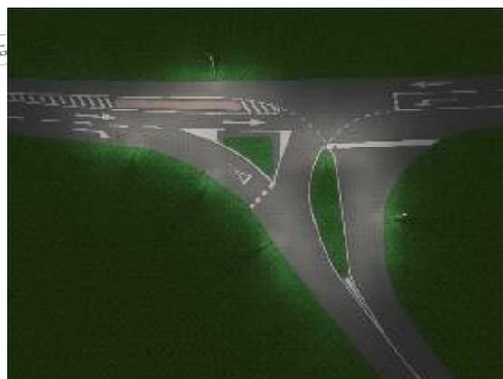
Figure 41: Example of the placement of lamps for the lighting of denivelated islands in an intersection
