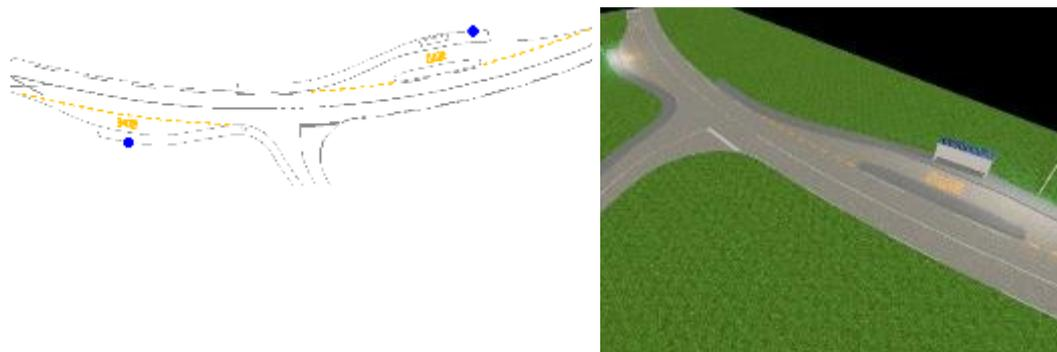
Figure 22: Example of a lamp installation for lighting bus stops outside settlements with a denivelated island
