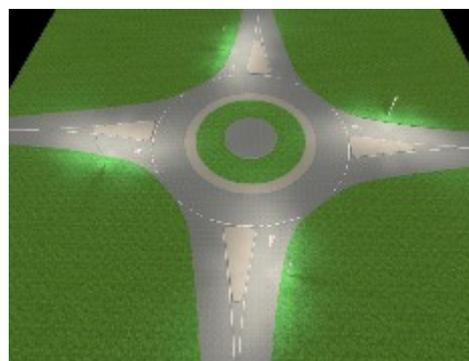
Figure 34: Example of the placement of lamps for lighting a roundabout without pedestrian crossings
