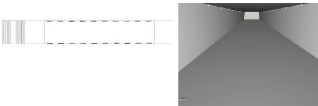
Figure 16: Example of the placement of lamps to illuminate underpasses under e.g. railway tracks
