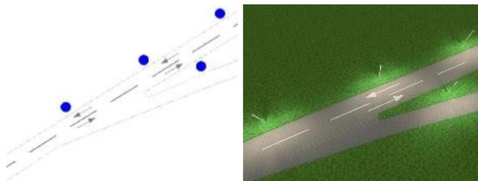
Figure 19: Example of the placement of lamps for the lighting of the long-distance road junction
