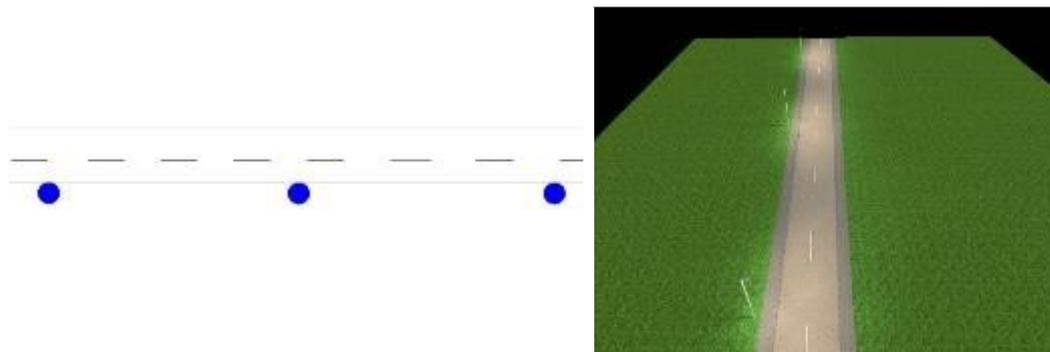
Figure 12: Example of placing lamps on one side of the road to illuminate pedestrian areas on the uncongested part of the road in a settlement
