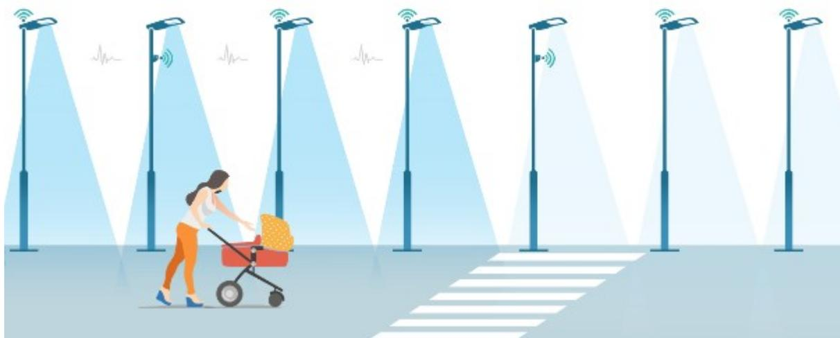
Figure 52: Demonstration of the operation of smart (dynamic) lighting, where appropriate conditions are ensured with regard to the presence of road users by means of sensors and communication between the lamps and the control station
