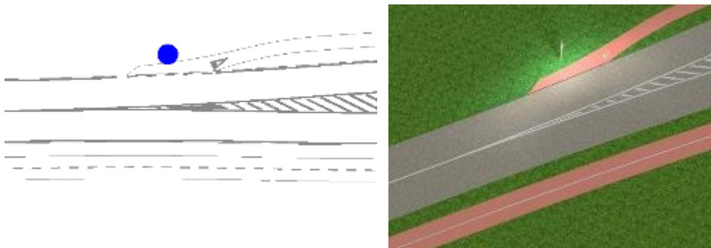
Figure 43: Example of the location of lights to illuminate the area where motor and cycle traffic intersect
