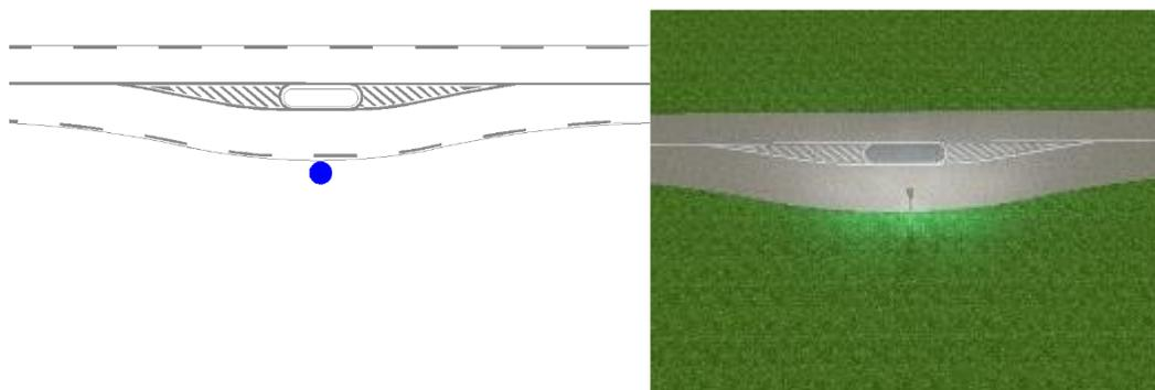
Figure 42: Example of placement of lights for the lighting of a denivelated island to offset the axis of the directional carriageway from one side of the road
