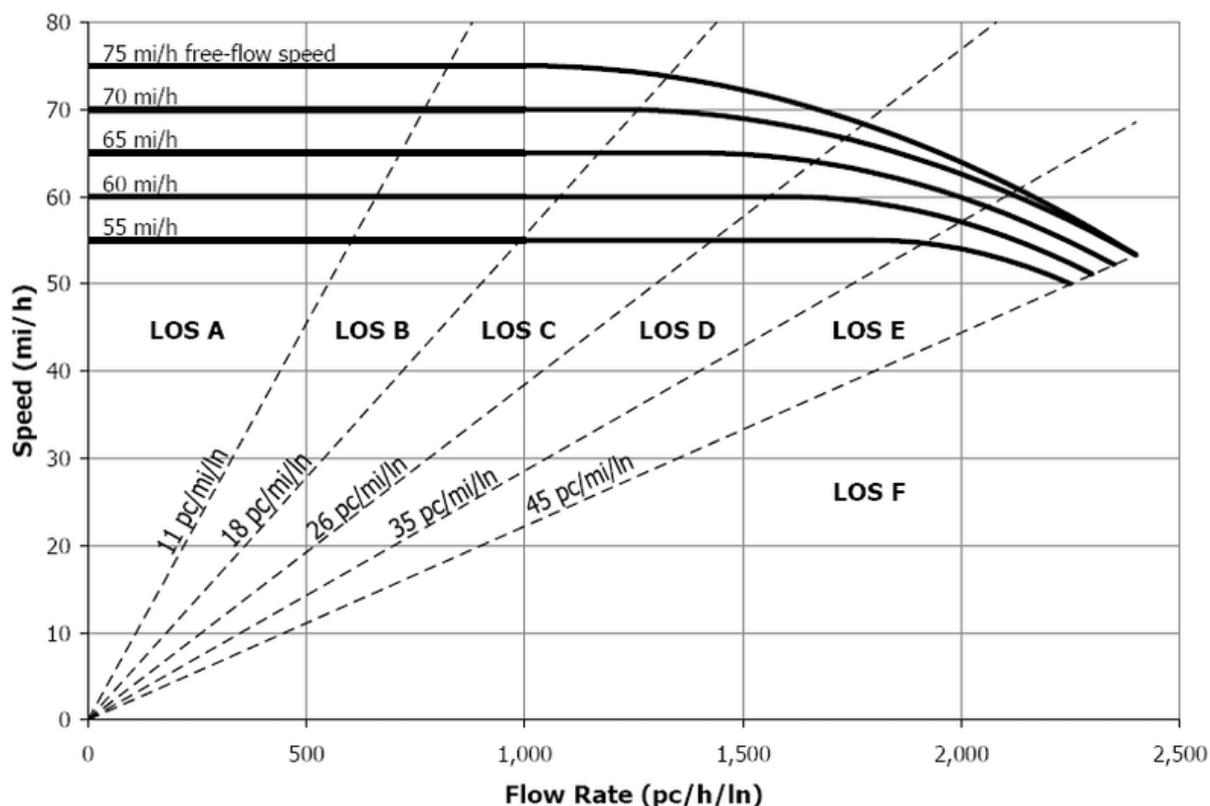
Figure A.3: The dependence of the limit flow on the free flow speed.
