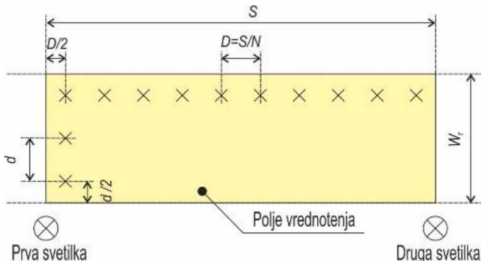
Figure 47: Measuring grid when measuring illuminance
