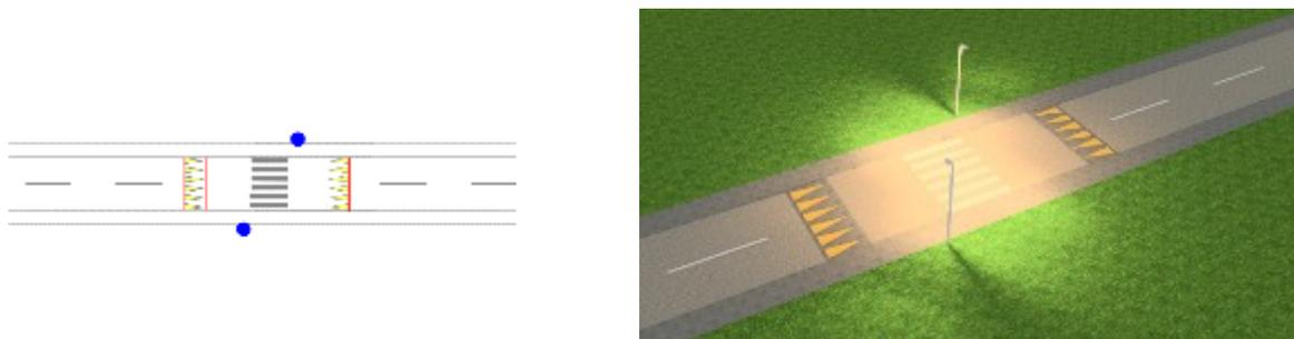
Figure 39: Example of the placement of lamps to illuminate the ramp of trapezoidal shape with a pedestrian crossing on the uncongested part of the road within the settlement
