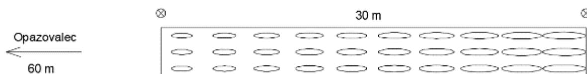
Figure 44: Size of the measurement point surface when measuring luminance with a suitable instrument
