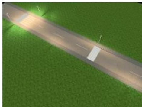
Figure 40: Example of the placement of lamps to illuminate the ramp of trapezoidal shape with a pedestrian crossing on the congested part of the road within the settlement
