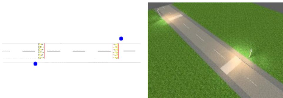
Figure 38: Example of the placement of lamps to illuminate the ramp of trapezoidal shape without pedestrian crossing on the uncongested part of the road within the settlement
