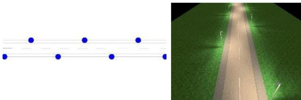
Figure 15: Example of placing lamps on both sides of the road to illuminate carriageway and pedestrian areas on the congested part of the road in a settlement
