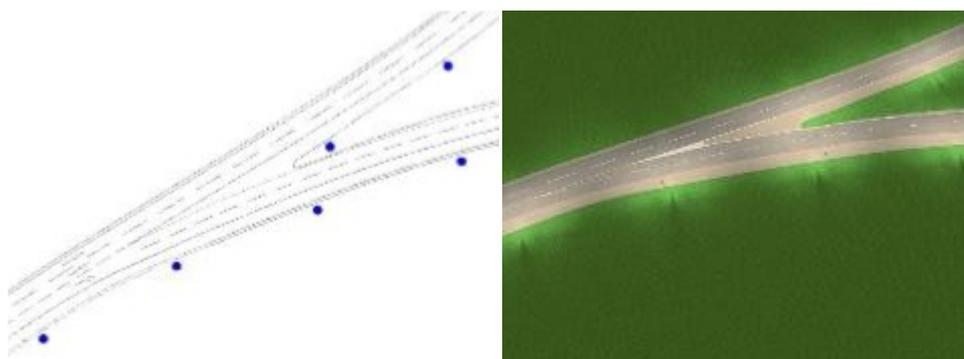
Figure 17: Example of the placement of lamps for the lighting of the motorway junction
