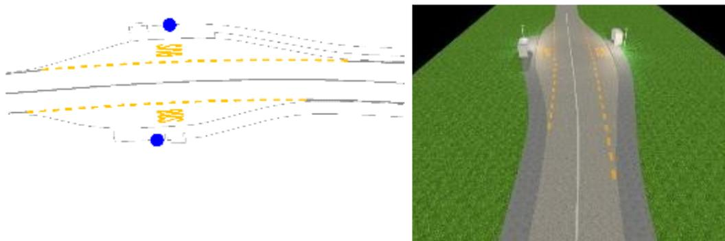
Figure 26: Example of lamps to illuminate opposite bus stops outside the carriageway on a road outside a settlement
