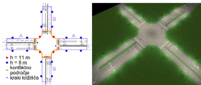
Figure 33: Example of the placement of lamps for the lighting of intersection with more than three classified lanes
