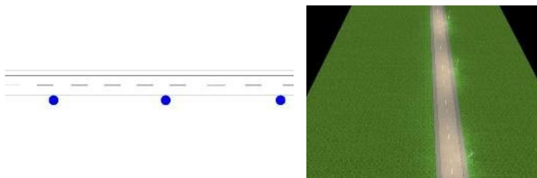
Figure 14: Example of placing lamps on one side of the road to illuminate carriageway and pedestrian areas on the congested part of the road in a settlement
