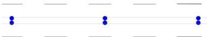
Figure 10: Two-sided central installation of lamps
