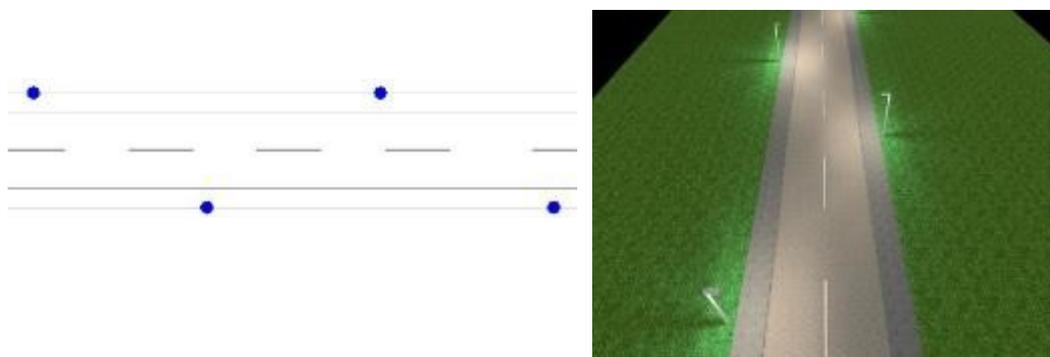
Figure 13: Example of placing offset lamps on both sides of the road to illuminate pedestrian areas on the uncongested part of the road in a settlement
