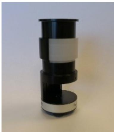
Figure 49: Meter for measuring semi-cylindrical illuminance
