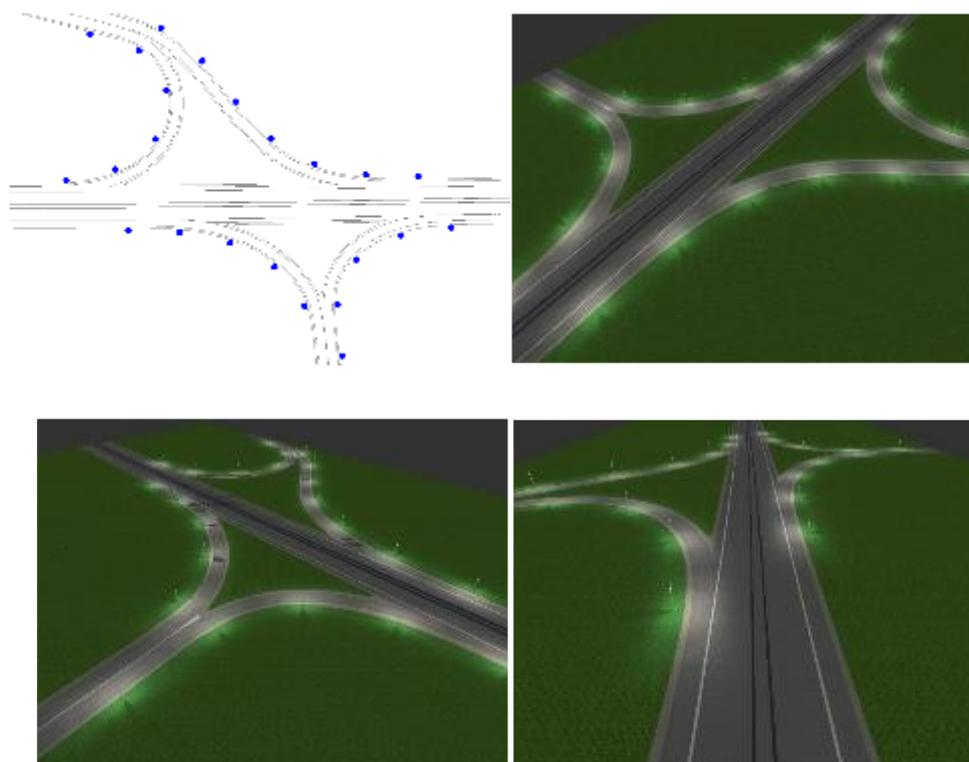
Figure 21: Example of the placement of lamps to illuminate the entry and exit on a motorway or expressway
