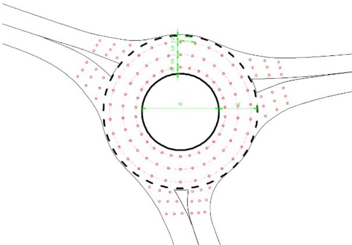
Figure 48: Example of a measuring grid when measuring illuminance at a roundabout
