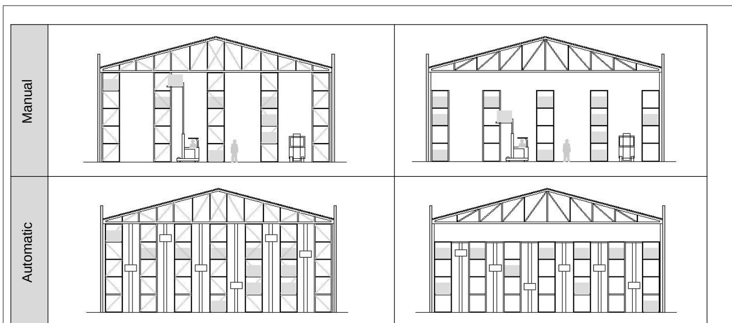
Figure 4.1. Classification of storage systems using metal shelves
