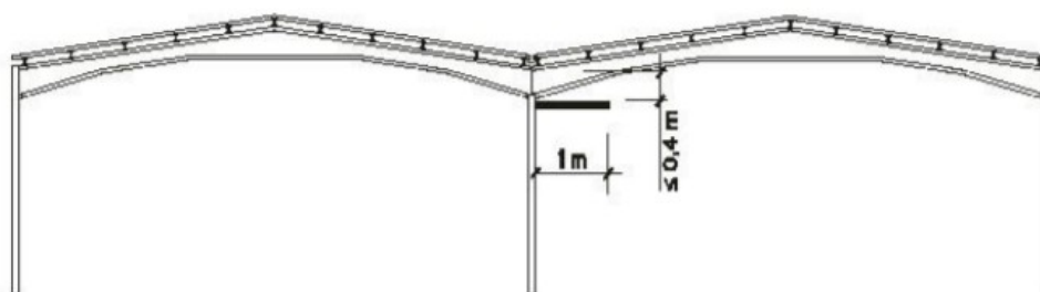
Figure 2.14: Compartmentalisation on deck by means of barrier under the cover.
