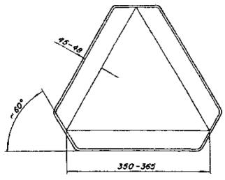
b) Shall be placed at the rear of the vehicle, pointing upwards and directed to the rear.
