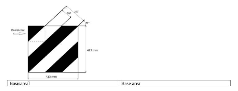
(3) The dimensions of each marking shall comply with the measures in the examples below. The figures only show the marking on one side: Form A
