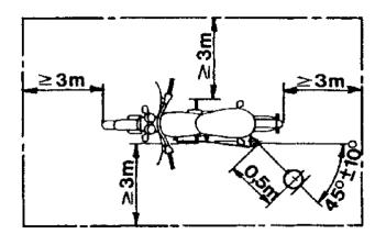
Microphone position and minimum measurement spots.
