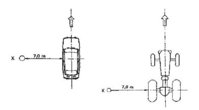
The sound pressure is measured from the centre of the vehicle, though, in the case of a tractor, next to the rear axle.
