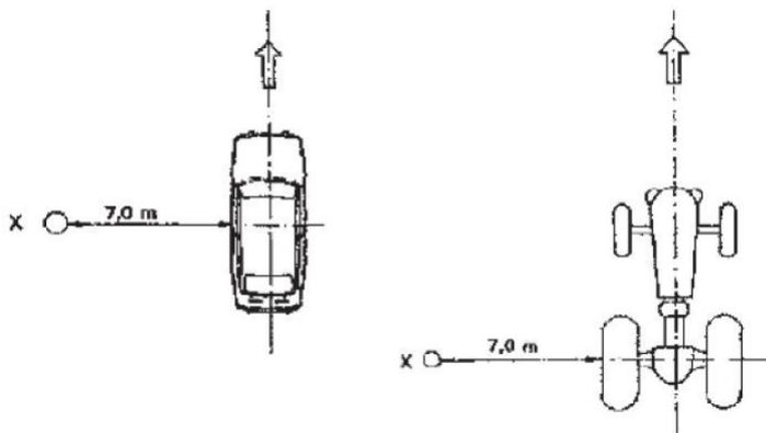
The sound pressure is measured from the centre of the vehicle, though, in the case of a tractor, next to the rear axle.
