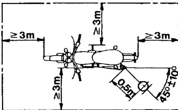
Microphone position and minimum measurement spots.
