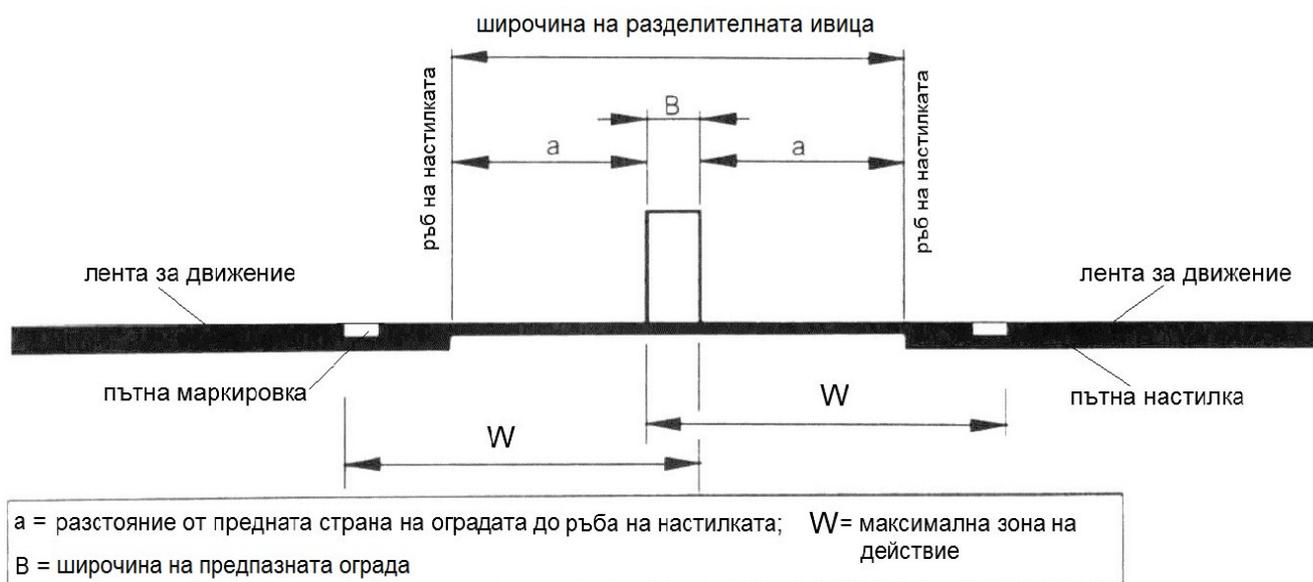
**Figure 15. Two-sided road restraint system located in the axis of the dividing strip**
