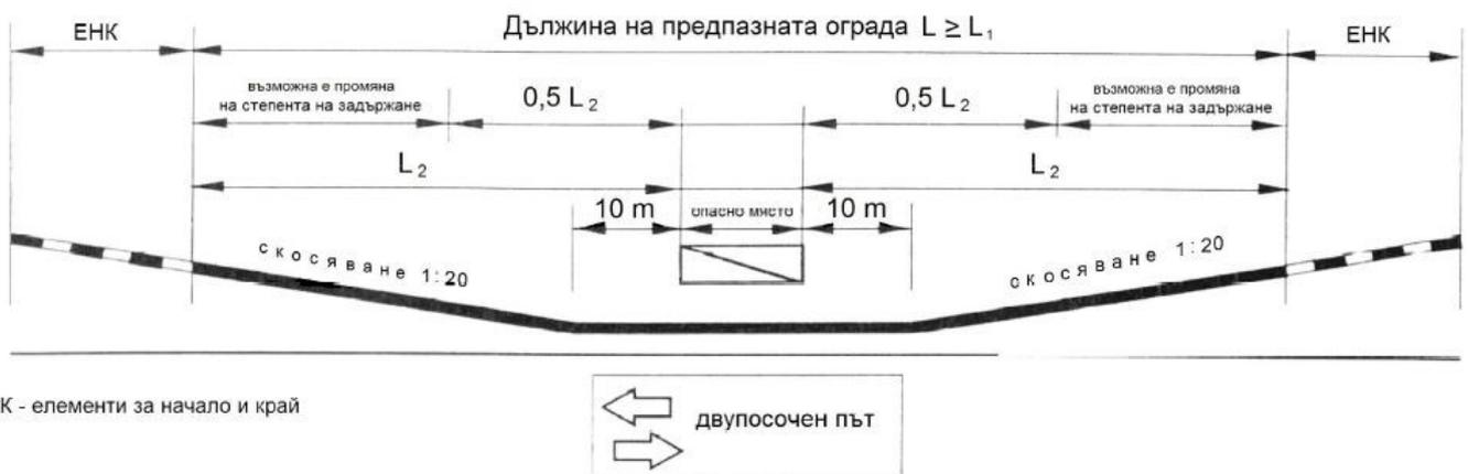
Figure 6. Minimum length of a road restraint system executed by two-sided bevelling before and after a hazardous location on a two-way road
