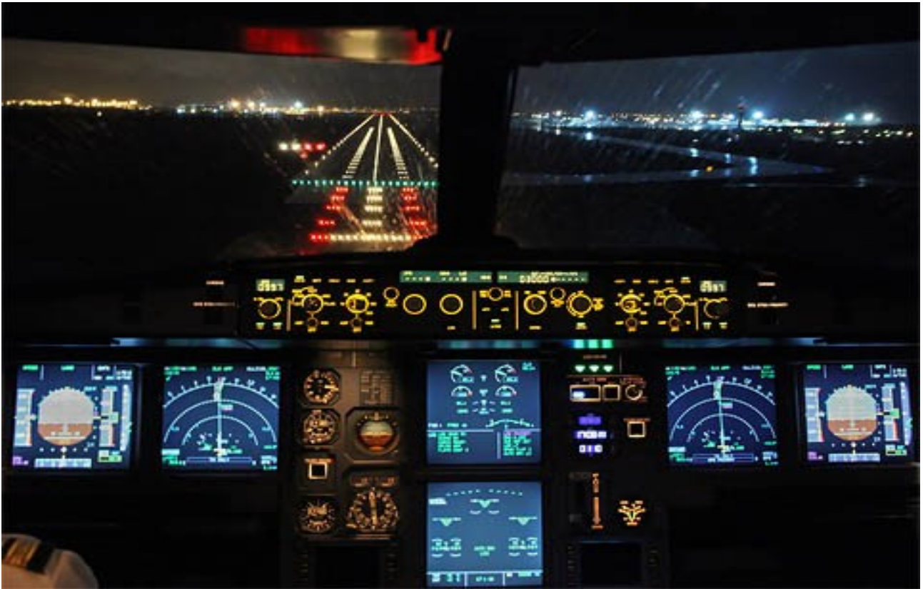
Figure 1 – The border and axis marking lights of the runway as seen from the aircraft cockpit
