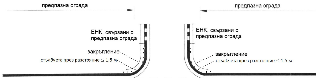
Figure 9d Interruption of a safety barrier with round-ups and ESE
