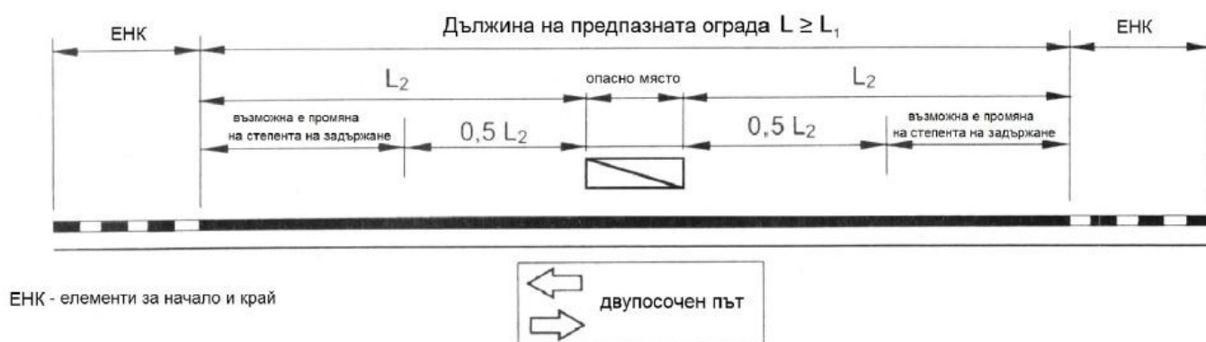
Figure 4. Minimum length of a road restraint system on a two-way road
